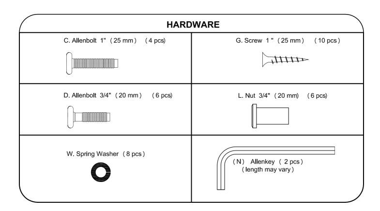
Make sure the bolts are tightly locked against the washers during assembly. (Please add an extra ½ revolution to all the bolts when using spring washer after tightening)
